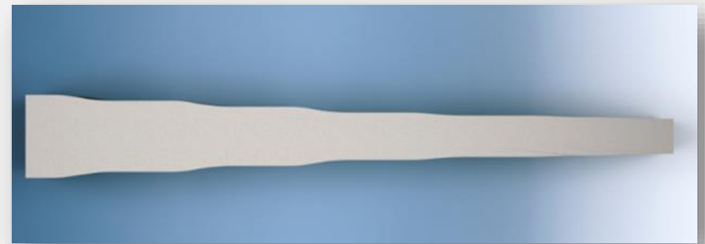
Multi-stage rectangular wind tunnel with stabilization sections
