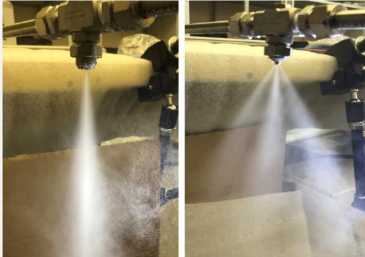
two types of air nozzles have been investigated
