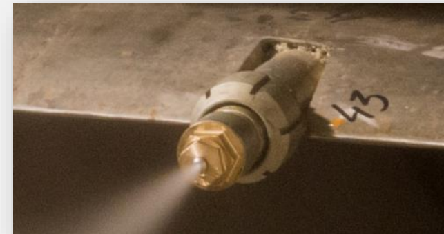
SU12J SS nozzle adapted to the AHT SD water spraying manifold
