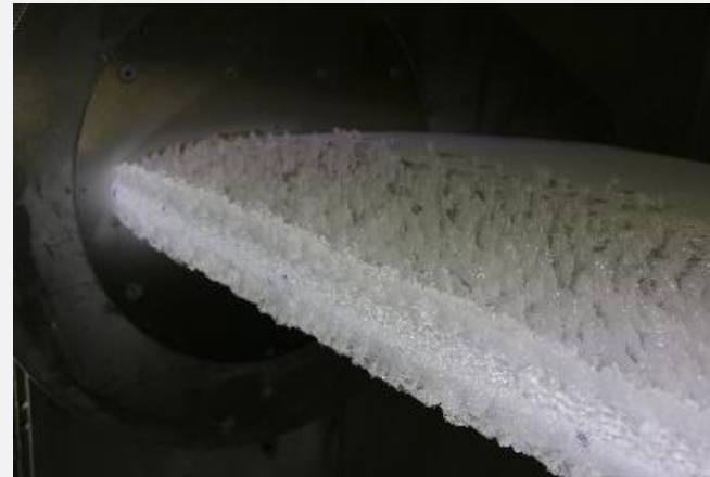
Figure 27: Photograph of FZRA ice shape on NACA0012 wing section
