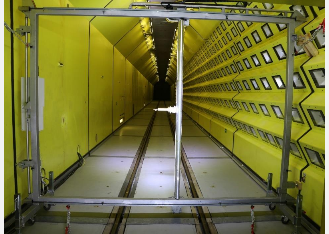
Figure 19: DLR Nevzorov Probe mounted on traversing system in the RTA IWT
