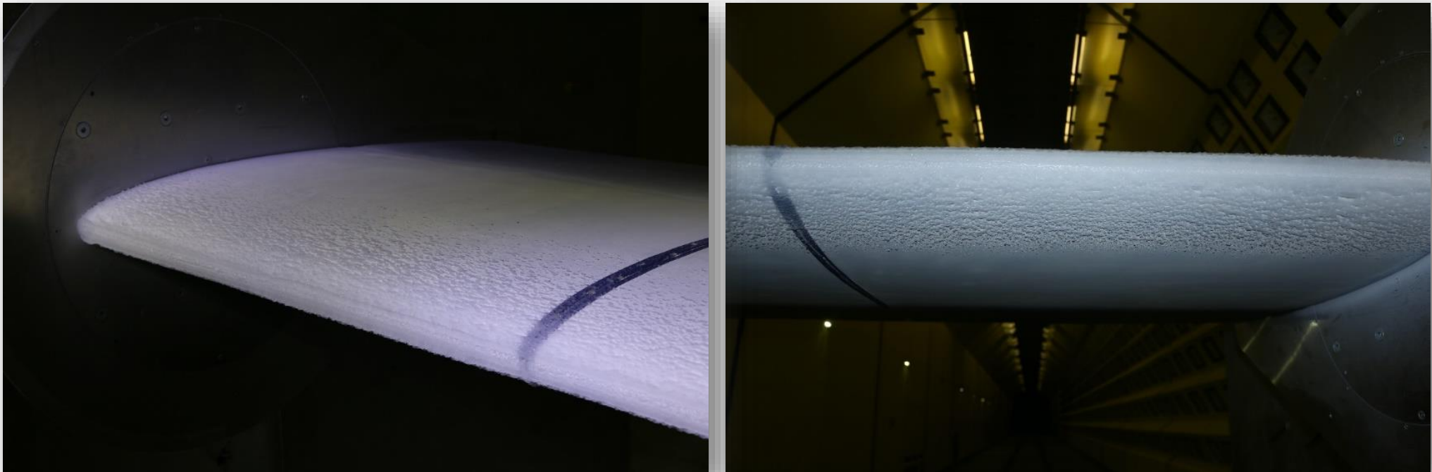
Figure 25: FZDZ MVD > 40 \mu\text{m} , ice accretion on NACA0012 wing section
