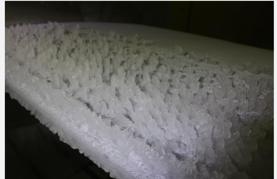
Figure 1: FZRA MVD > 40 \mu m ice accretion on NACA0012 wing section, at RTA IWT
