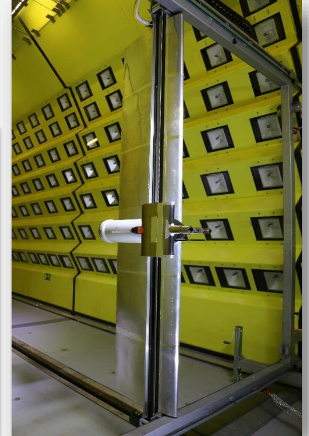
Figure 17: DLR CAPS Probe mounted on traversing system in the RTA IWT
