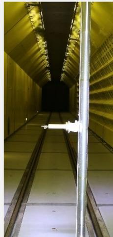
DLR CAPS probe (left) and DLR Nevzorov Probe (right) mounted on traversing system in the RTA IWT
