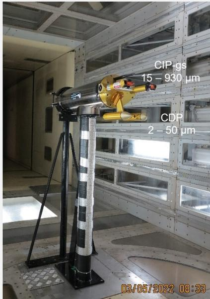
DLR CCP (left) and CIRA PDI-4D (right) were installed in the main test section configuration of the CIRA-IWT.
