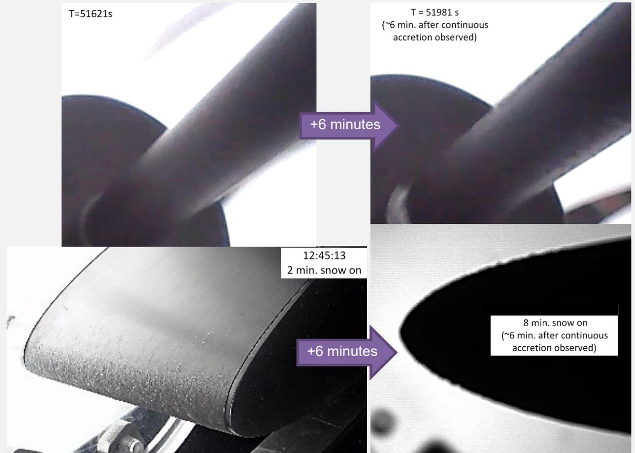
Comparison of flight F06-1 round bar (top) to airfoil accretion TP883 (bottom)
