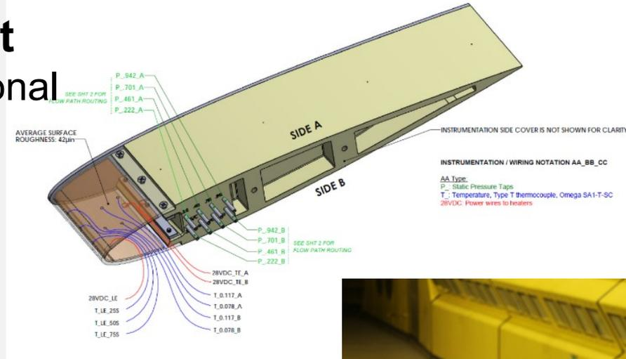
Figure 10: Schematic of NACA0012 test article, provided by NRC
