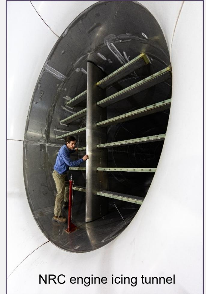
NRC engine icing tunnel
