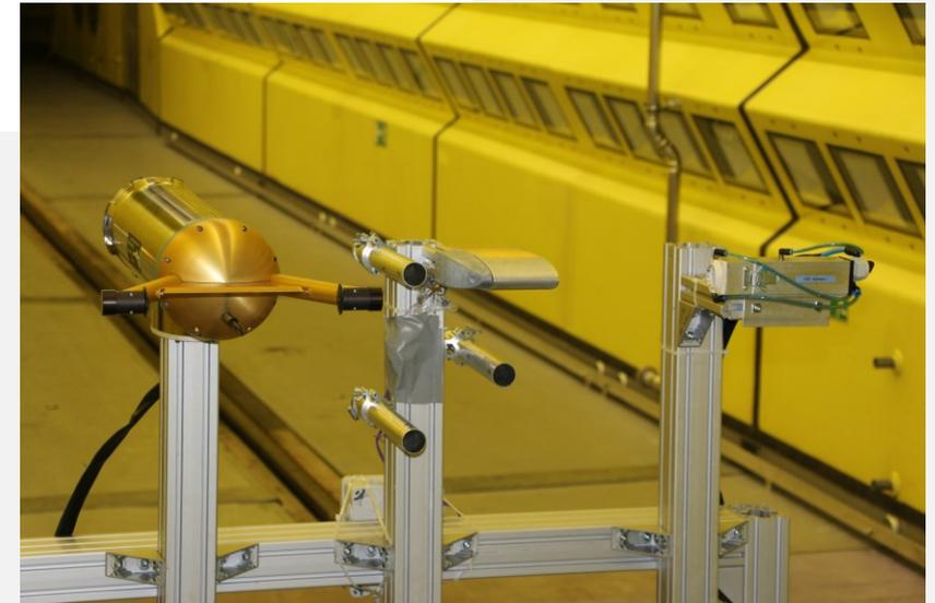
Figure 11: Test setup of the NACA0012 accretion tests, PIP (left), test article and ICCs (center) and camera (right)
