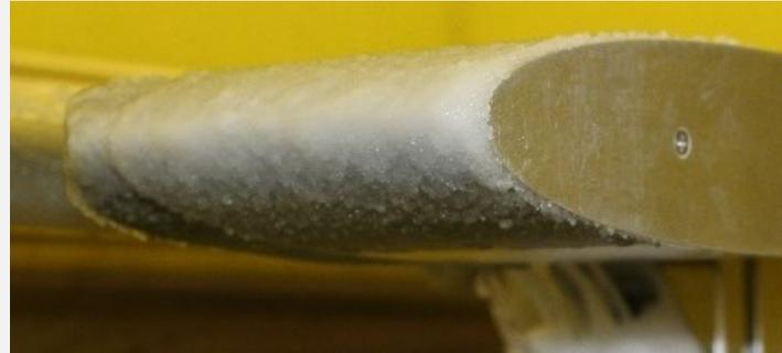
Figure 16: Photograph of snow accretion on NACA0012 airfoil, RUN9 - wet snow (SF480) at 40 m/s
