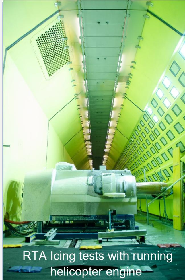
RTA Icing tests with running helicopter engine
